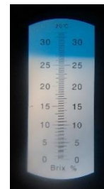
Left to Right: 1) Ripe Red Bourbon coffee cherries to be collected at the end of the harvest on Mesias's farm. 2) Mesias looking through the BRIX refractometer to see the TDS (total dissolved solids), or sweetness level on his cherries. 3) The reading on the BRIX refractometer signaling about 27 - a very good score for coffee fruit.
