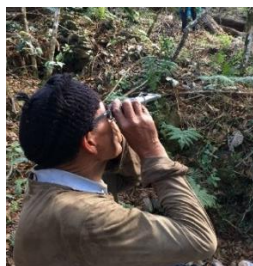
Left to Right: 1) Ripe Red Bourbon coffee cherries to be collected at the end of the harvest on Mesias's farm. 2) Mesias looking through the BRIX refractometer to see the TDS (total dissolved solids), or sweetness level on his cherries. 3) The reading on the BRIX refractometer signaling about 27 - a very good score for coffee fruit.
