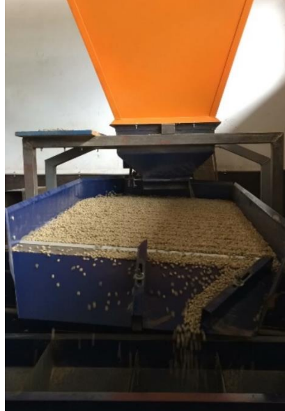
Gravity sorting machine separating beans based on weight and density.
