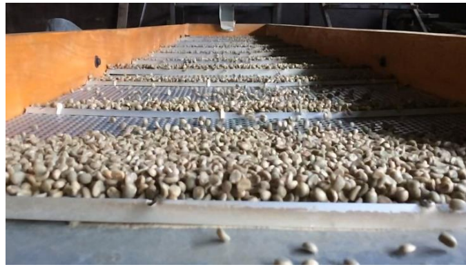
Above From Left to Right: 1) Dry mill in which all the coffee was milled, 2) Screen sorter separating bean size, 3) Gravity table sorter separating beans by density.
