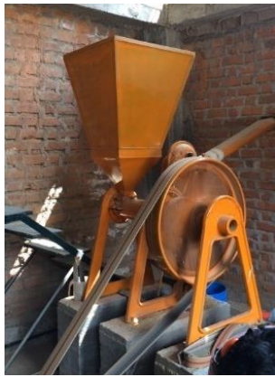
Above From Left to Right: 1) Dry mill in which all the coffee was milled, 2) Screen sorter separating bean size, 3) Gravity table sorter separating beans by density.
