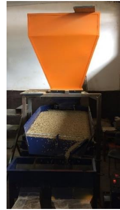
Above From Left to Right: 1) Dry mill in which all the coffee was milled, 2) Screen sorter separating bean size, 3) Gravity table sorter separating beans by density.
